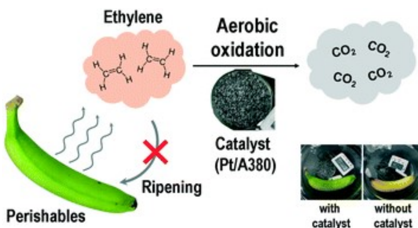
Figure 2. SiO 2 -supported platinum catalysts for perishables preservation [34] .
