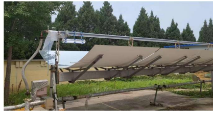
Figure 2. New type of trough solar photovoltaic composite device.
