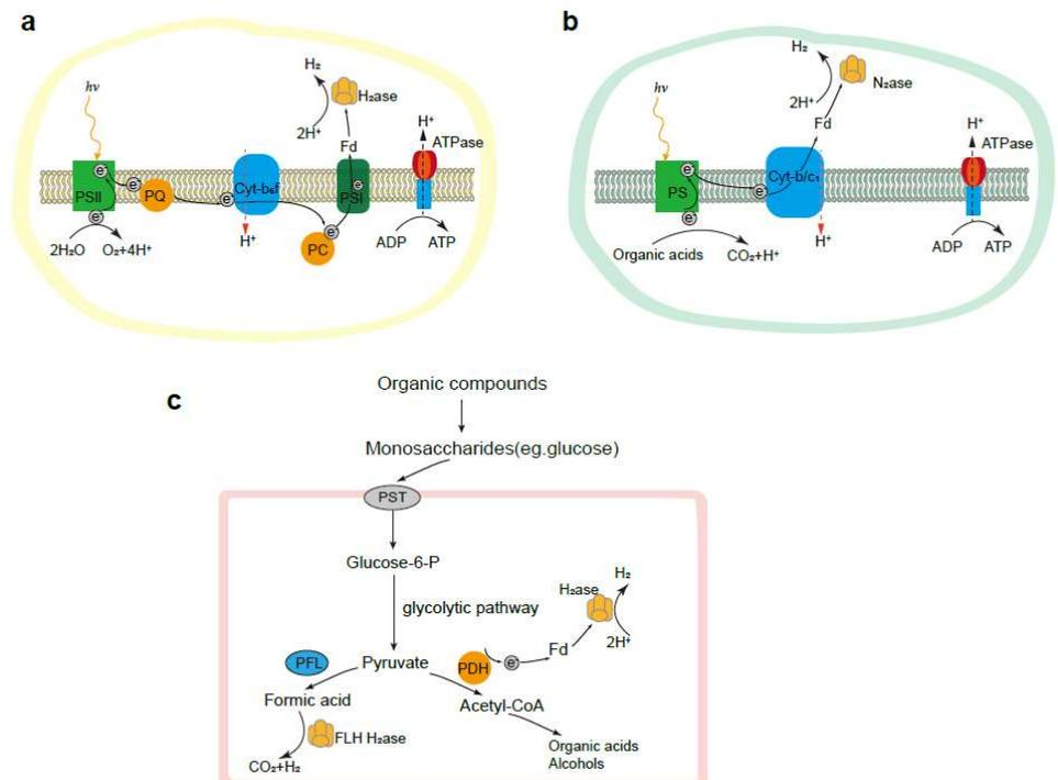
**Figure 1.** Metabolic pathways in basic biohydrogen-producing system: **(a)** biophotolysis, **(b)** photo-fermentative, and **(c)** dark fermentative.
