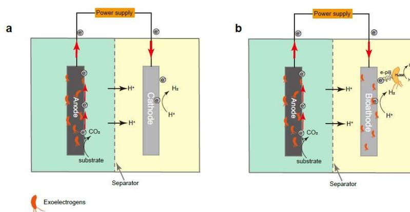
**Figure 3.** Schematic diagram for hydrogen production: **(a)** non-biocathode MEC and **(b)** biocathode MEC.
